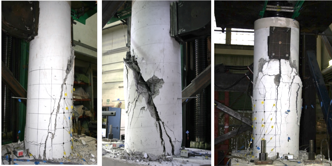
Figure 5.5 Specimen S1 final state: southeast face (left), southwest face (center), and north face (right)
