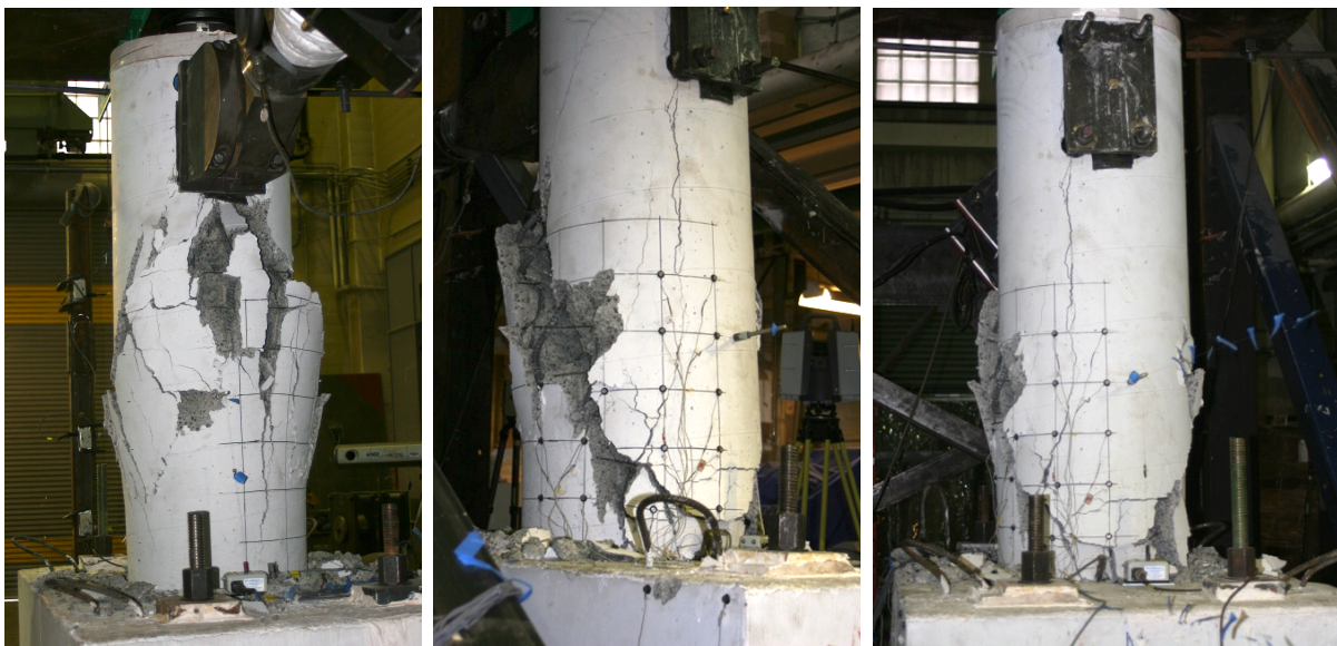
Figure 5.6 Specimen S3 final state: southwest face (left), northeast face (center), and north face (right)
