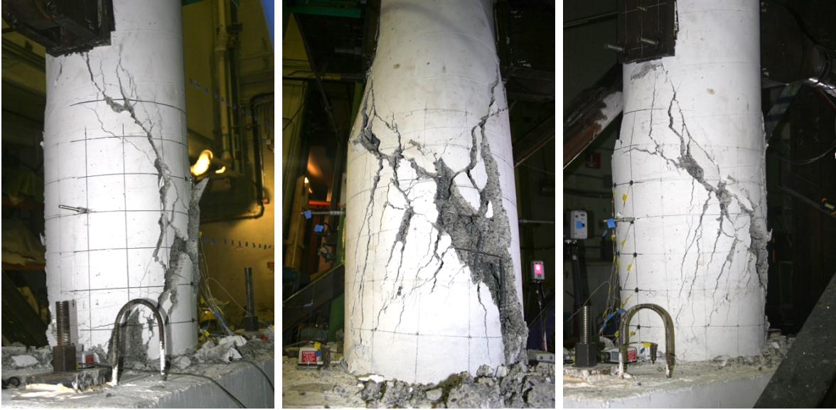
Figure 5.7 Specimen S6 final state: southeast face (left), west face (center), and northwest face (right)
