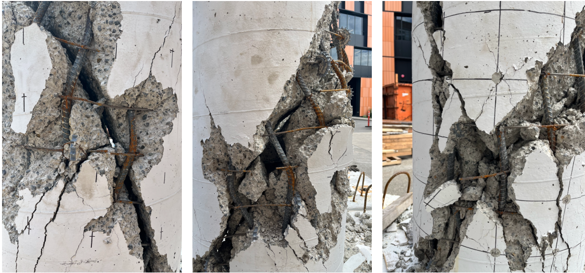
Figure 5.3 Opened hoops observed per specimen: S1 (left), S3 (middle), and S6 (right)
