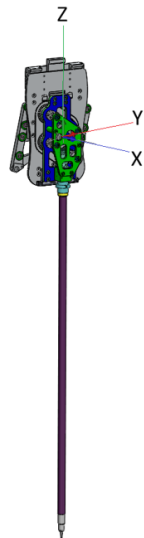
Figure 2.2: CAD models of the Raven for first three joints. CAD derived mass of links 1, 2, and 3 are 0.503Kg, 0.753Kg, and 0.407Kg, respectively.
