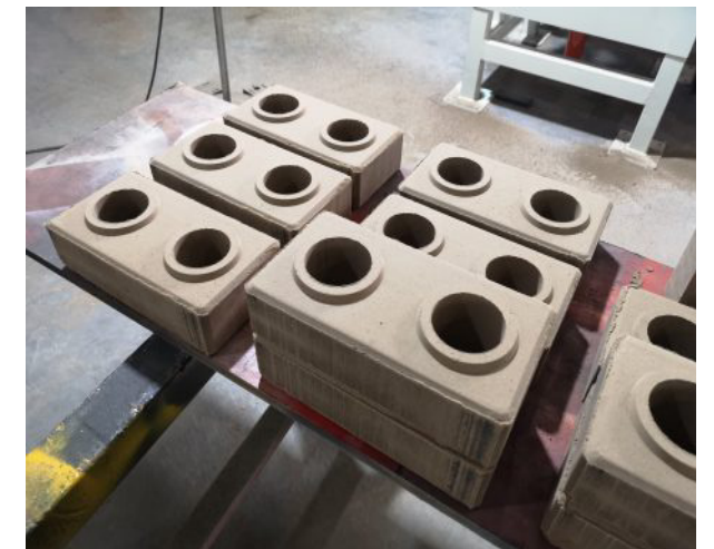
Figs. 49-50 (top to bottom): ByA Block-making machines, "Automatic hydraulic press (top) with CEB products (bottom), Jan. 2019.
