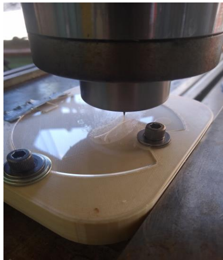
Figure 33. Machining of the flow channel
