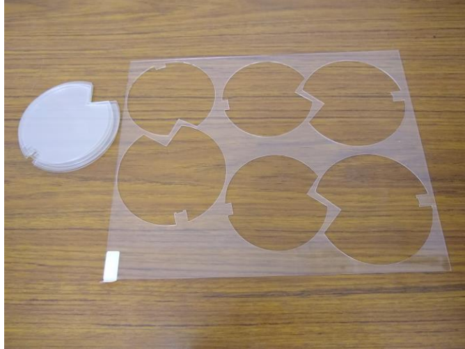
Figure 31. Cutouts laser cut from an acrylic sheet
