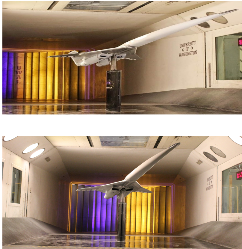
Figure 5.3: Wind Tunnel Model with Low Boom Nose Installed
