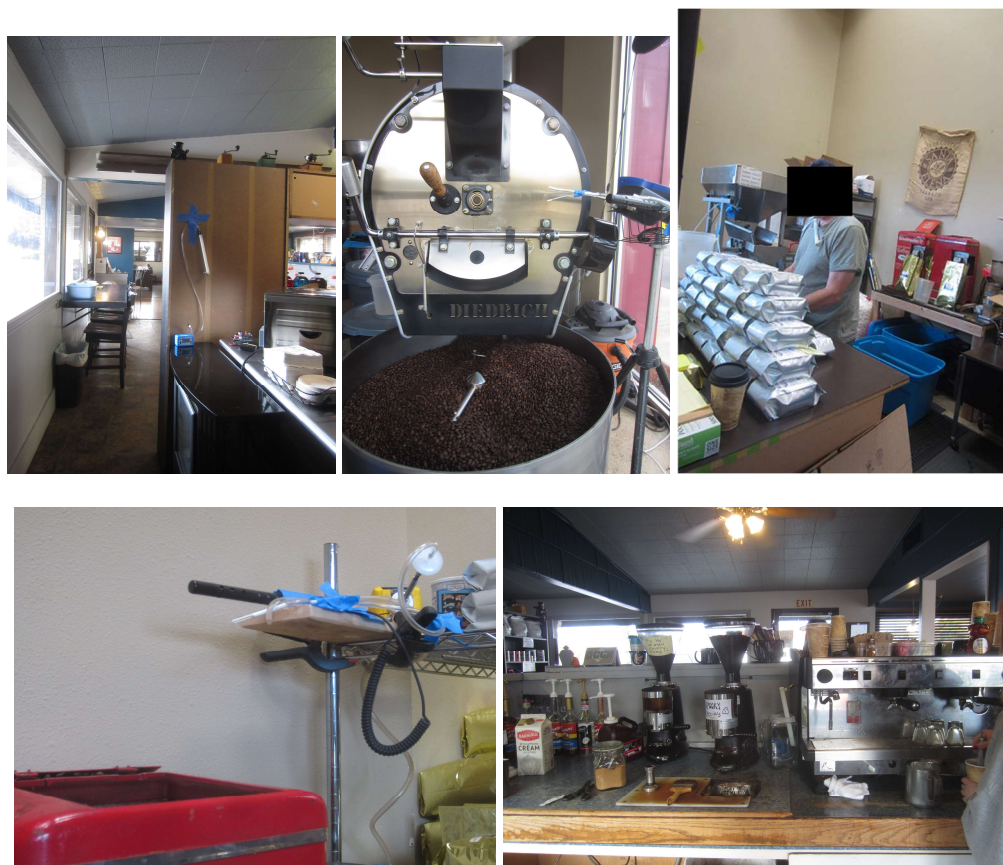
Figure 3. Images illustrating where area air samples were collected in the roastery and café. Area sampled in the café included behind the café shelves to capture the background concentrations of alpha diketones in the facility (top left) and on the barista counter adjacent to the espresso grinder (bottom right). Areas sampled in the roastery were above the cooling tray of the roaster (top middle), above one of two Grindmaster grinders (bottom left), and adjacent to the chute of the hopper (bottom left) where roasted ground or whole beans drop into the machine's funnel that fills the bags.
