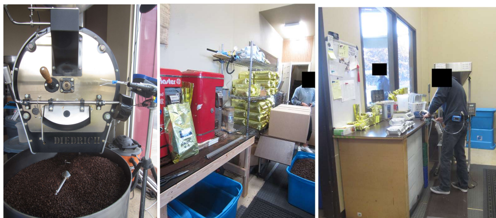
Figure 2. Images of the Diedrich IR-12 roaster (left) used in the roasting room, the Grindmaster grinders (center) used to grind roasted coffee and the shelves where packaged coffee is stored to off-gas, and a worker using the Logical Machines S5 hopper to package roasted beans.
