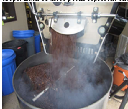
Figure 5b. After the roasting is completed, the beans are automatically dropped from the roasting chamber into the machine’s cooling chamber to cool before further processing.
