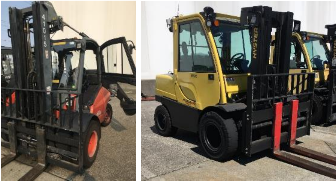
Figure 2.2. Forklifts tested: Forklift A with mast-based vibration damping system (left) and Forklift B without the mast-based vibration damping system (right)
