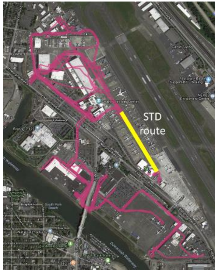
Figure 2.4. A map showing GPS coordinates of forklift operating routes (pink) and the selected common route (yellow)
