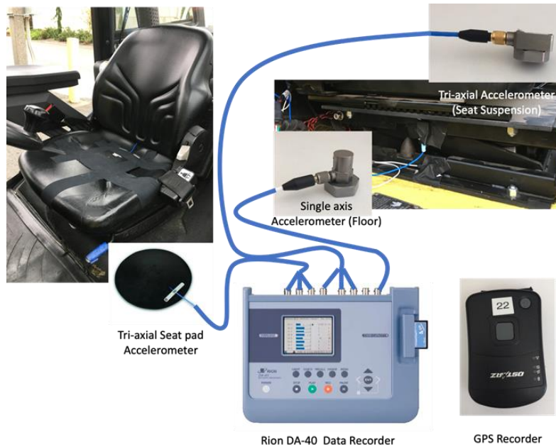
Figure 4.2. Whole-Body Vibration data collection instrumentation with three accelerometers
