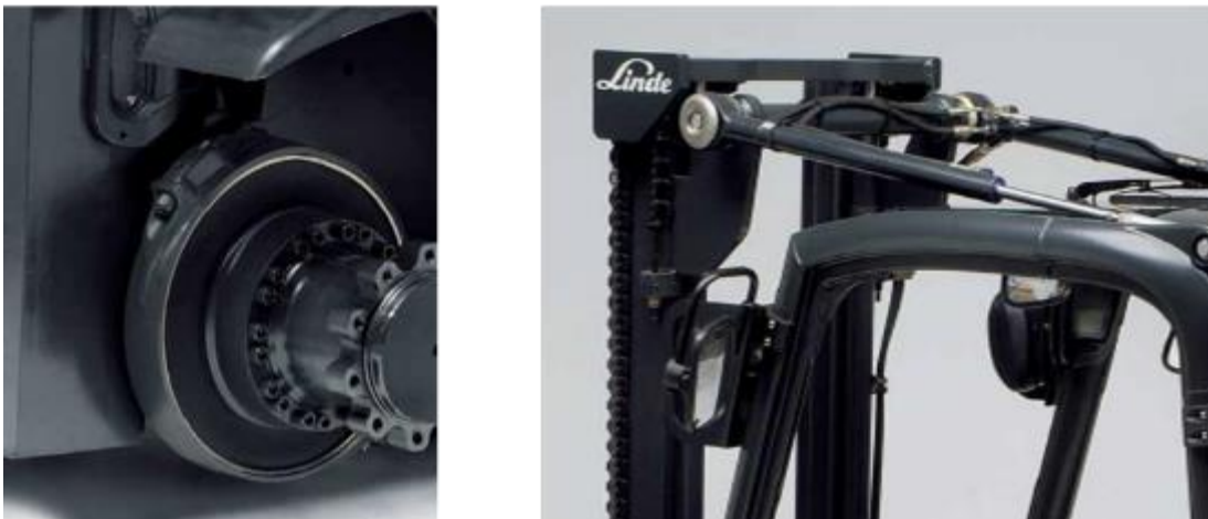
Figure 2.1. Front Axle mounted on the mast (left) and a hydraulic shaft connected between mast and cabin of the forklift (right) (Linde Material Handling, n.d.).
