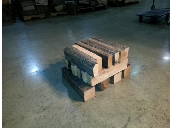
Figure 3.4: White oak fuel used in one of the experiments.
