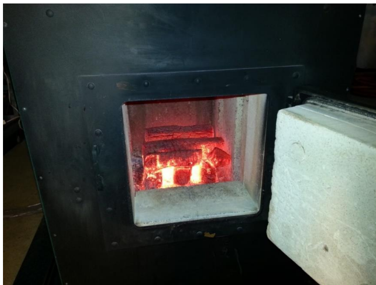
Figure 3.2: White Oak burning in the biomass furnace.
