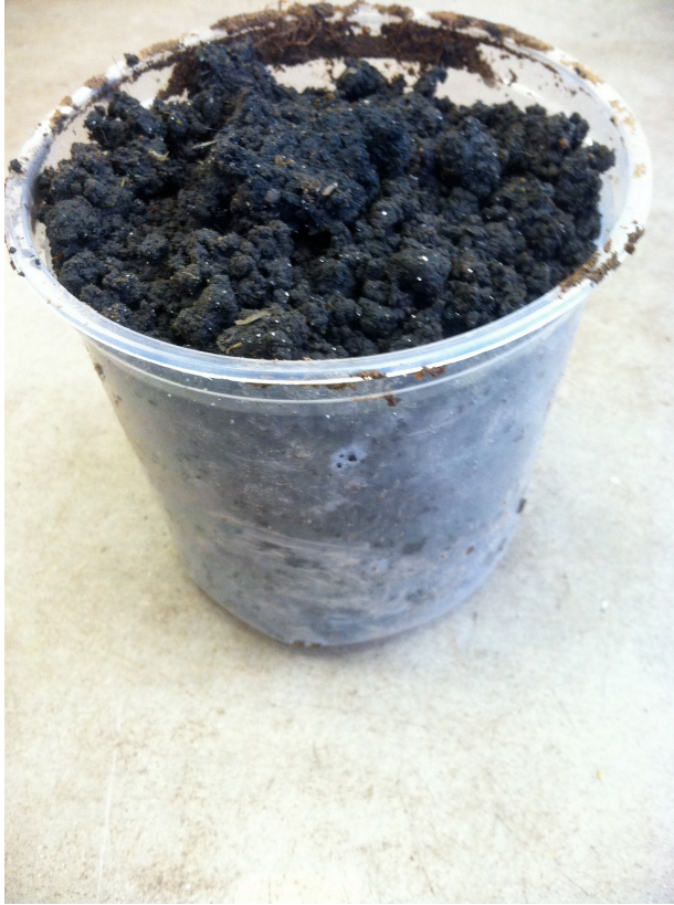
Figure 2.3a Class B cake biosolids used to amend soils for Cake Rate 1 and Cake Rate 2 treatments. Class B cake was provided by King County. Application rates were equivalent to 20 \text{ Mg ha}^{-1} (Cake Rate 1) and 40 \text{ Mg ha}^{-1} (Cake Rate 2). Cake was 22% solids with metal concentrations ( \text{mg kg}^{-1} ) of Cd, Cu, Pb and Zn of 2.5, 500, 30 and 900, respectively, as reported by King County.
