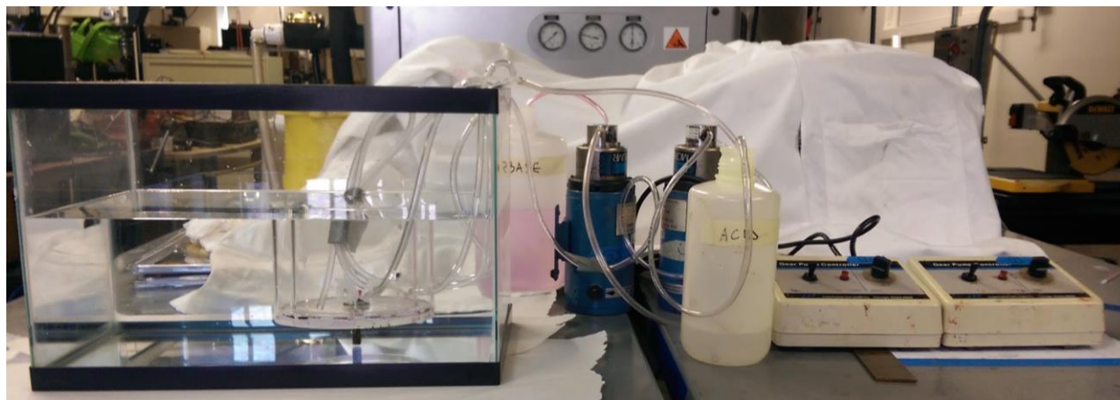
Figure 4.3: Image of the experiment setup for the liquid flow mixing test
