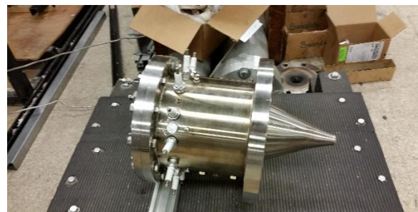
Figure 2.4. Fully assembled RDE with expansion nozzle
