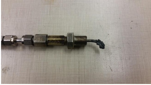
Figure 3.12. Partially melted pitot tube used in the combustor region.
