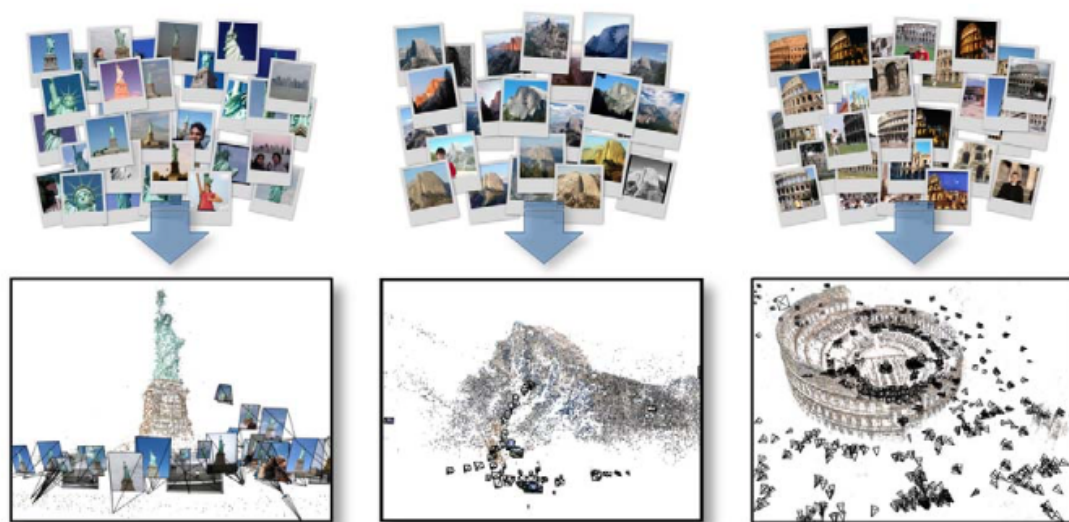
Figure 1.2: Snavely et al.’s 3D reconstructions of landmarks from Internet photo collections using a Structure-from-Motion technique. The goal of this work is to provide the experience of being at those places.
