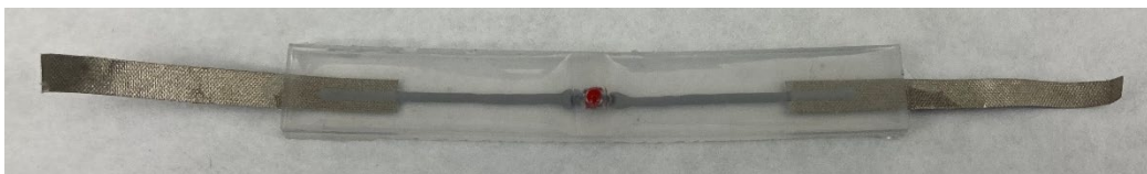
Figure 6 Tensile specimen with mounted LED
