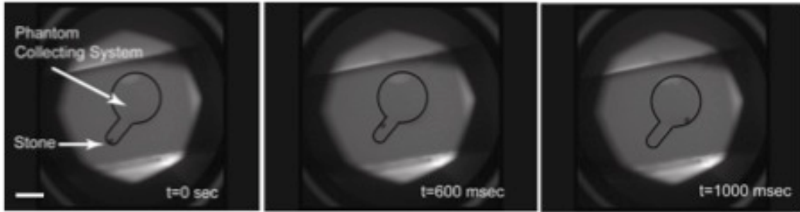
Fig.4.5. Fluoroscopic monitoring of an artificial stone that was repositioned from the lower pole into the collection system of a kidney phantom. Displacement of the stone was seen immediately after the application of focused ultrasound and the total distance traveled was approximately 1 cm. The estimated velocity magnitude was 1 cm/s
