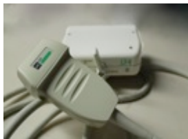
Fig.2.2. left: The Verasonics ultrasound engine (VUE) and right: the ATL L7-4 probe.
