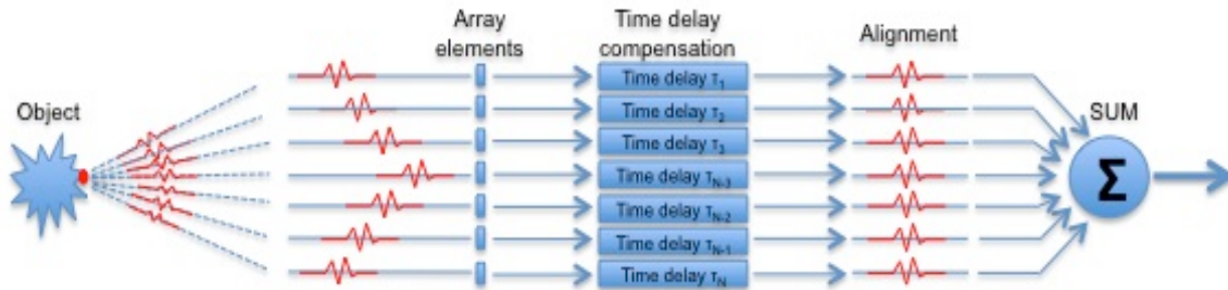
Fig.2.8 Flow chart of the conventional beamforming technique. As shown in the figure, when applying ultrasound to the object, the ultrasonic echoes scatter back. Because of the geometry of the receiving array, those echoes arrive at different elements of the transducer at different times. By matching the beamformer time delays (different \tau in the flow chart) to the signal propagation delays of the acoustic field, all signals scattering from the same location on the object can be aligned. Then, the amplitude of the coherent wavefront can be enhanced by summing the aligned signals together.
