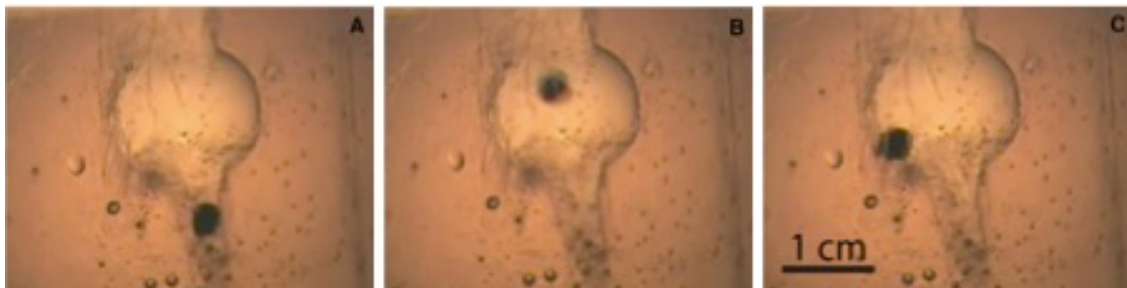
Fig.4.7. Video photography monitoring of an artificial stone (a) before, (b) during, and (c) after delivering focused ultrasound.
