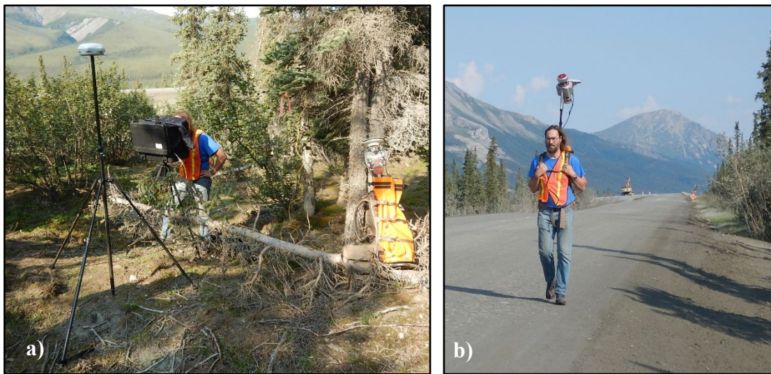
Figure 2.3. LiDAR data collection: (a) setting up the LiDAR system; (b) acquiring LiDAR data along the old Dalton Highway embankment in July 2018.
