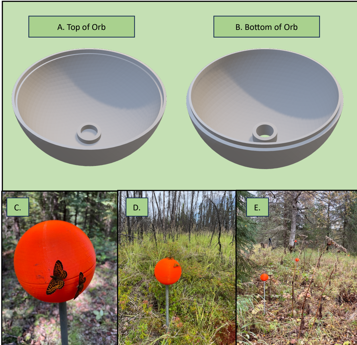
Figure 15: 3D model used to print target orbs. The orbs have a diameter of 145 mm. On the left, A is the top of the orb, it has an indentation on the inside rim and a circle in the center which the conduit fits into. On the right, B is the bottom of the orb, it has a matching indentation on the outside of the rim which locks with the top rim, and an open circle in the center which is used to mount the orb on the conduit. The 3D models were designed by Jonathan Batchelor ( JonathanBatchelor.org ). On the bottom, C, D, and E, show photos of the orbs being used in Alaska. Photos were taken by Rachel Deiningger. Orange generally works well for target orb color because it is easy to find in a colored point cloud, making registering multiple scans and stitching them together easier.
