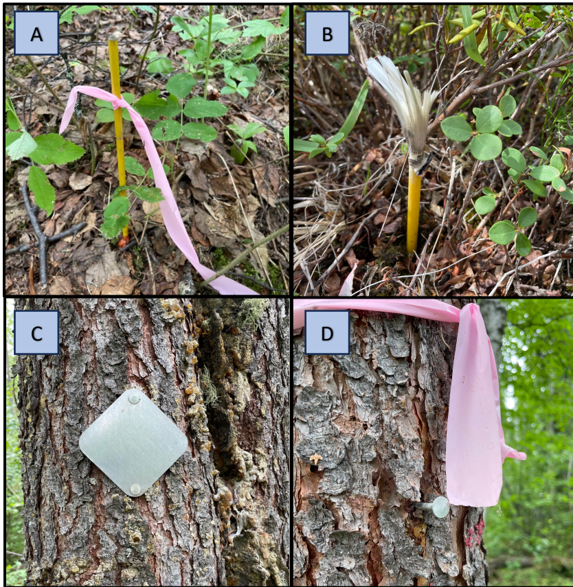
Figure 14: Pins and Witness Trees. A and B show pins used to mark the location of FIA plots. B is an example of a pin damaged in a fire. C and D show different markers used on witness trees, while C has a plaque, D is only just a nail. These are all examples of permanent monumentation used by FIA to set up and re measure plots. Photos taken by Rachel Deiningger
