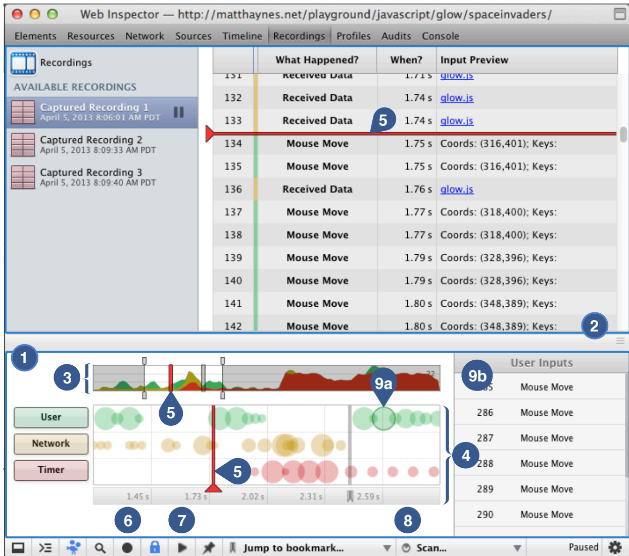
Figure 5.1: The Timelapse tool interface presents multiple linked views of recorded program inputs. Above, the timelines drawer (1) is juxtaposed with a detailed view of program inputs (2). The recording overview (3) shows inputs over time with a stacked line graph, colored by category. The overview's selected region is displayed in greater detail in the heatmap view (4). Circle sizes indicate input density per category. In each view, the red cursor (5) indicates the current replay position and can be dragged — Buttons allow for recording (6), 1× speed replay (7), and breakpoint scanning (8). Details for the selected circle (9a) are shown in a side panel (9b).
