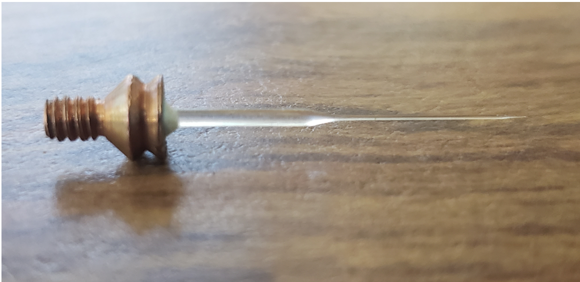
Figure 3.2: Fiber screw with broken fiber attached. The rod stock is 1 mm thick and pulled to 250 \mu\text{m} after the first stage of pulling.
