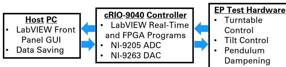
Figure 5.4: A flow diagram highlighting the main components of the torsion balance's DAQ system. Credit: Conner Gettings.
