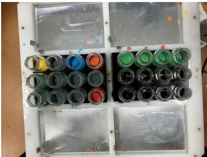
Figure 5.7: Experiment samples after a color mixing optimization campaign in which the objective was to make the greenish color on the right.
