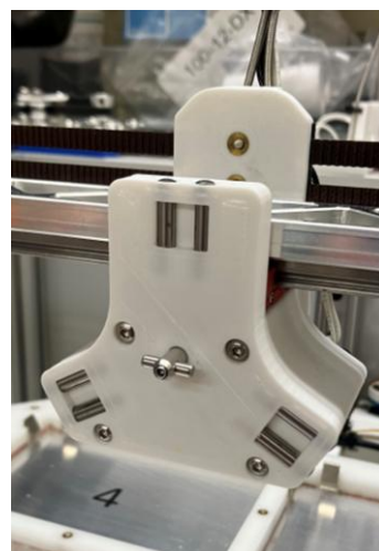
Figure 5.2: Close up of the tool changing head that enables Jubilee to swap tools on the fly.
