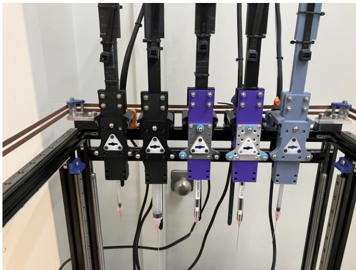
Figure 5.4: Five adapted Digital Pipette tools mounted on a Jubilee.
