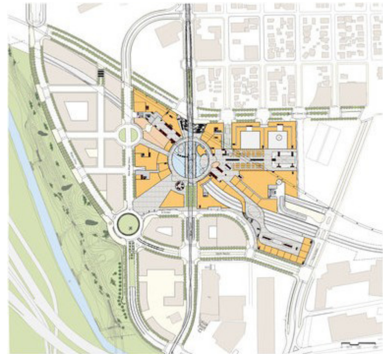
Figure 2.5 Houston Northern Intermodal Facility - Ground floor plan
