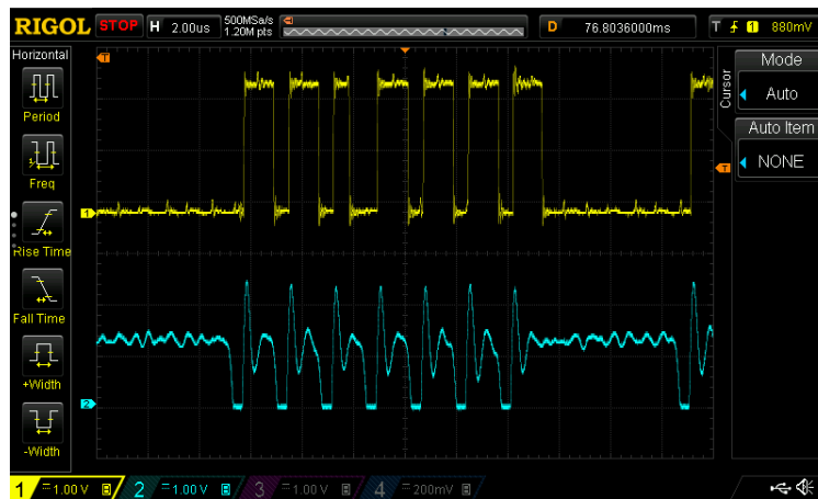
Figure 5.23: Implant receiving information frames at 576 kbps.
