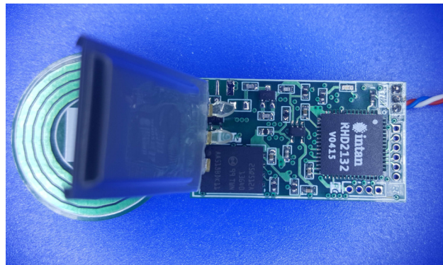
Figure 3.2: The "lollipop" optogenetic stimulation device.
