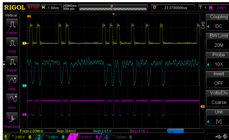
Figure 5.24: IrLAP information frame reliably transmitted at 2Mbps.
