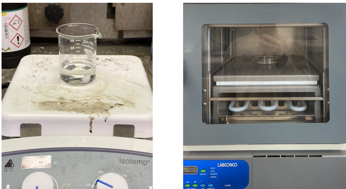
Figure 5, Acid Piranha Bath of Diced Silicon Wafer Fragments (left), subsequent Freeze-drying of Drop-Casted Wafers (right)
