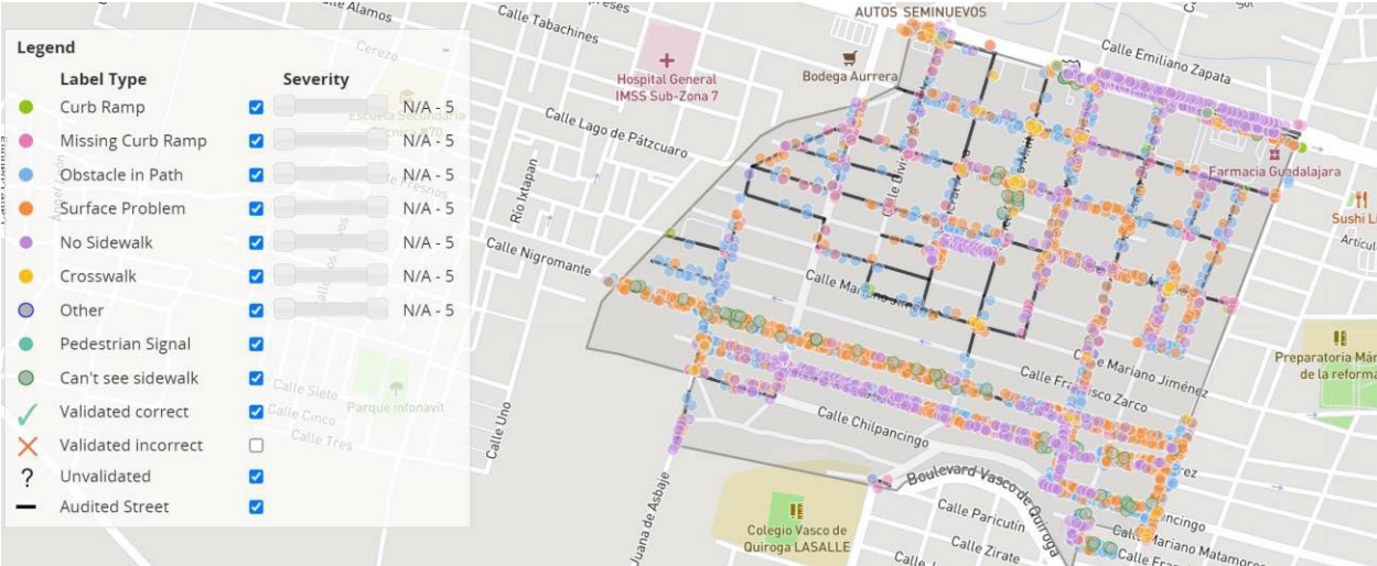
Figure 2.2 A map of our pilot deployment in La Piedad, Mexico. Each circle represents a geo-located accessibility label color-coded by label type. For example, orange is a “ surface problem ” and purple is “ no sidewalk. ” Thirty-five users have audited 8.3 miles of the 11.3-mile pilot neighborhood (73 percent), contributing 3,006 labels and 800 validations
