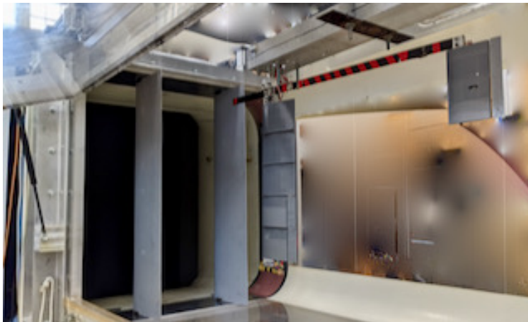
Figure 4.33: MARGE test-bed installed in U. of Washington 3 ft \times 3 ft wind tunnel.
