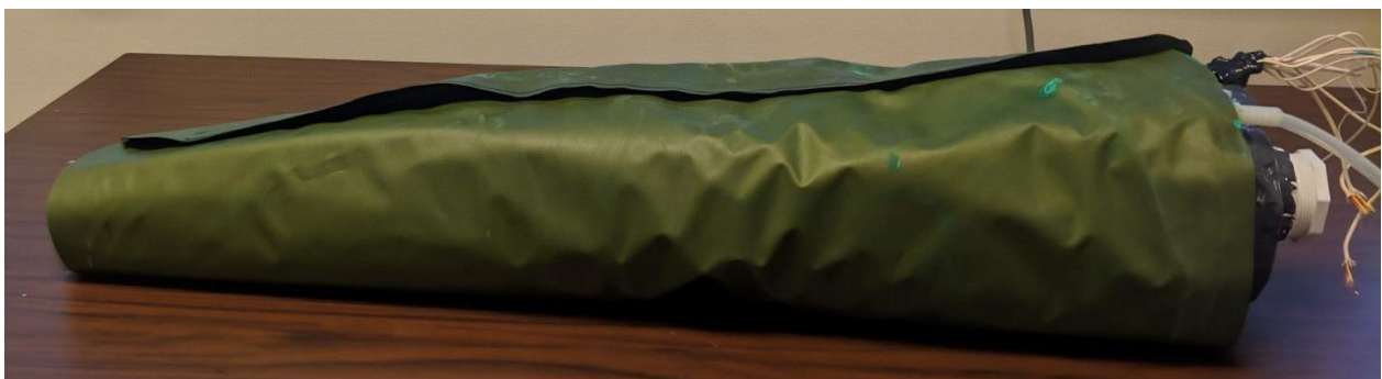
Figure 63: Cooling sleeve and air splint wrapped around the phantom
