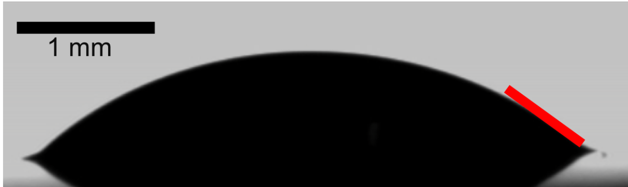
Figure 3-3: Example of a sessile drop on a surface, with the contact angle marked by a red line.
