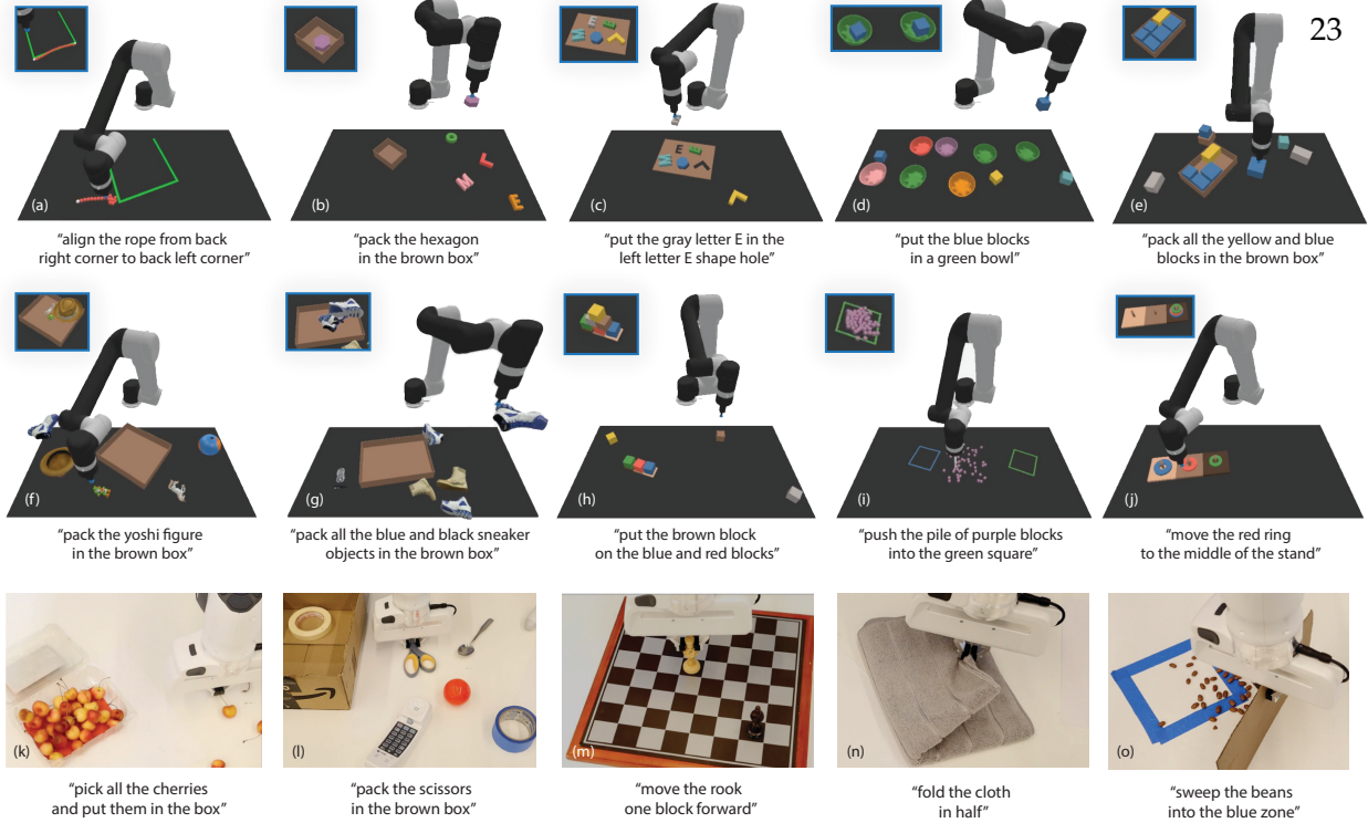
FIGURE 3.1: Language-Conditioned Manipulation Tasks. CLIPort is a broad framework applicable to a wide range of language-conditioned manipulation tasks in tabletop settings. We conduct large-scale experiments in Ravens [311] on 10 simulated tasks (a-j) with 1000s of unique instances per task. See Table 3.1 for challenges pertaining to each task. CLIPort can even learn one multi-task model for all 10 tasks that achieves better or comparable performance to single-task models. Similarly, we demonstrate our approach on a Franka Panda manipulator with one multi-task model for 9 real-world tasks (k-o; only 5 shown) trained with just 179 image-action pairs.
