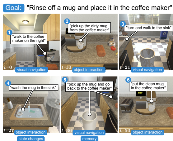
FIGURE 2.1: ALFRED Challenge . ALFRED consists of 25K language directives corresponding to expert demonstrations of household tasks. We highlight several frames corresponding to portions of the accompanying language instruction. ALFRED involves interactions with objects, state changes, and long-horizon planning.
