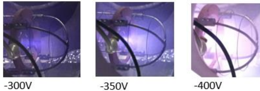
Figure 21. Plasma injection despite of spherical grid on anode at pressure of 44mTorr
