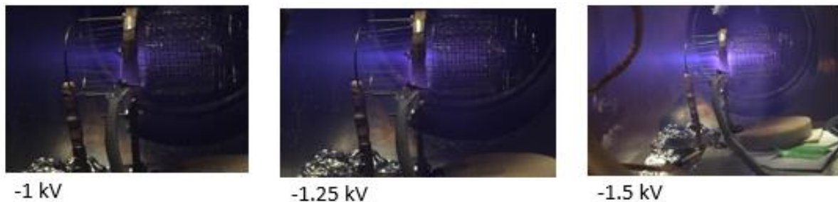
Figure 23. Plasma injection of 4 th version as cathode voltage increases
