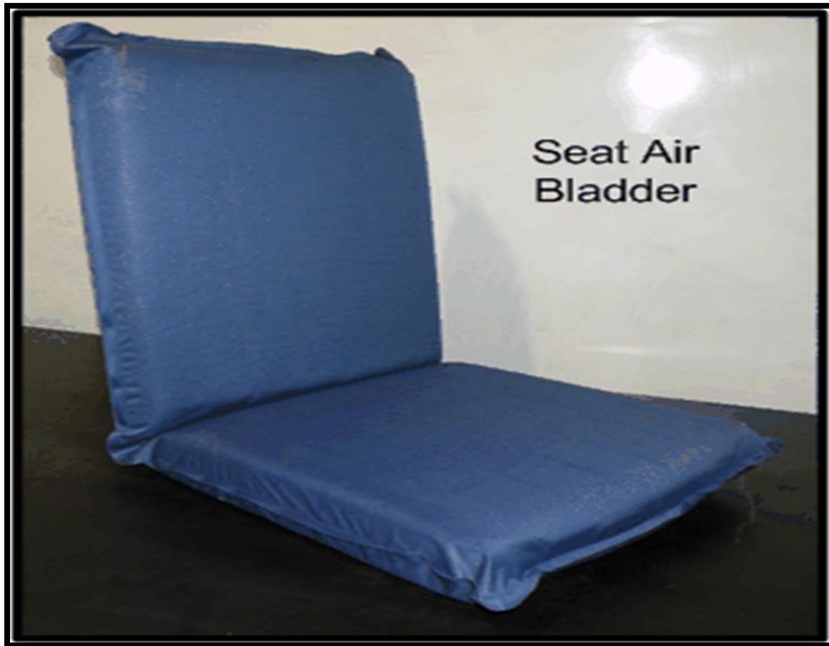
Figure 1. Whole-Body Vibration Exposure Intervention: A Ballistic Air-Filled Seat Pad
