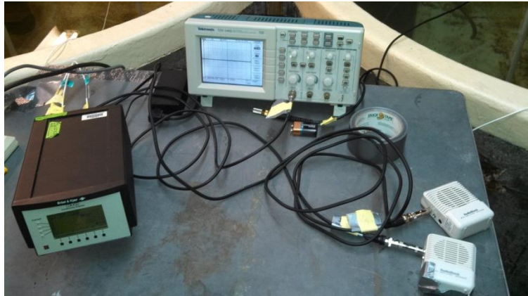
Figure 3. From left to right: B&K multi-channel conditioning amplifier, oscilloscope, and two portable speakers. The oscilloscope was used to measure peak-to-peak amplitude, wave period, and frequency at any given time.
