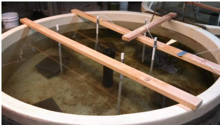
Figure 2. Photograph of experimental tank setup, specifically showing the hydrophone and male nest setup
