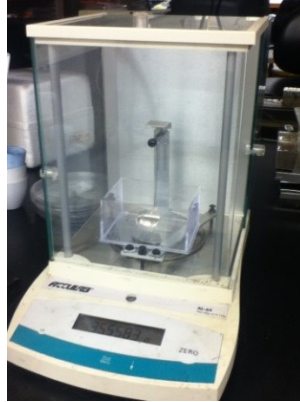
Figure 5-3 Setup for density measurement using Archimedes method.
