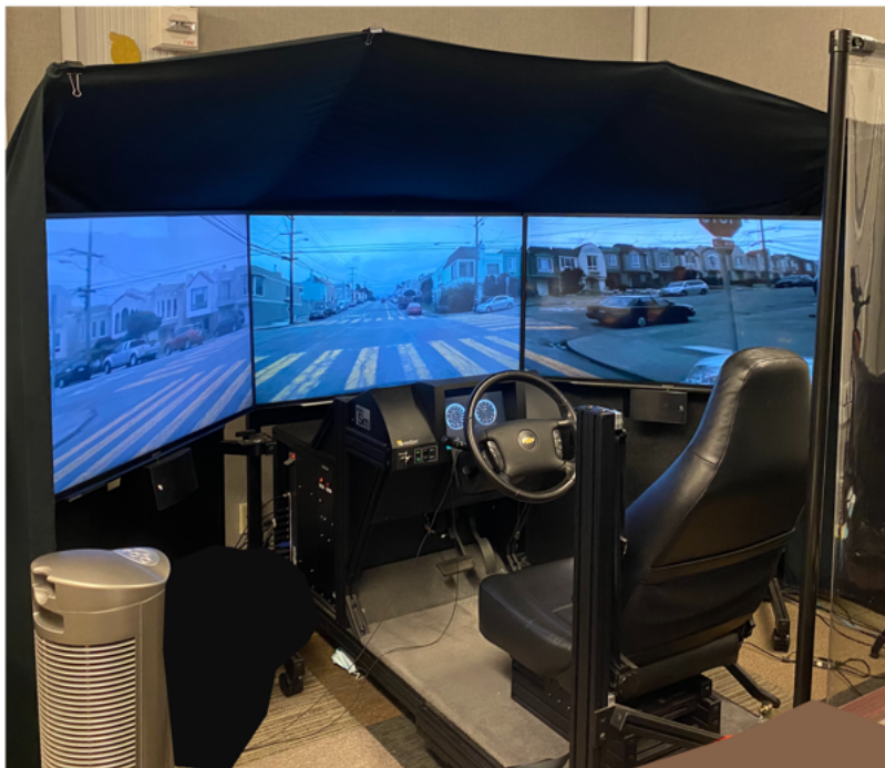
Figure 4.1: The driving simulator of HFSM lab showing a scenario across three displays
