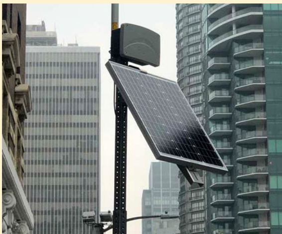
Figure 4: Deployment of curb availability sensors on a passenger load zone and commercial vehicle load zone in Seattle, WA. 274 curb parking availability sensors were installed on commercial vehicle load zones and passenger load zones
