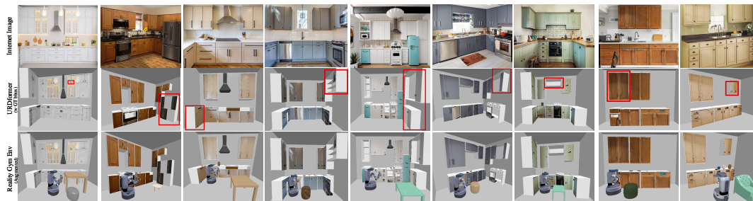
Figure 29: Generated Kitchen Scenes: Examples of kitchen scenes predicted by URDFormer from internet images given labeled bounding boxes. Examples of failure parts are highlighted in red boxes.
