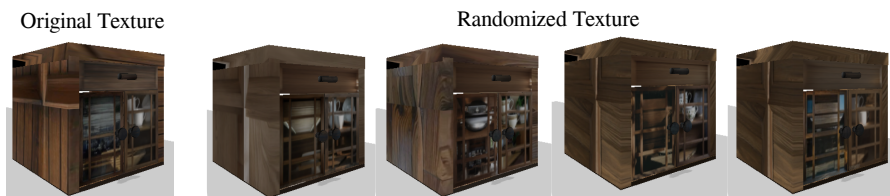
Figure 62: We randomize the texture of the object using stable diffusion to cover the distribution of the real world
