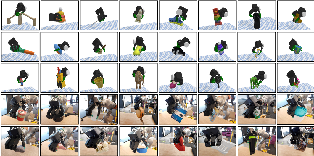
Figure 20: Qualitative results on unseen objects in simulation and in the real world. The top 3 rows shows the successful examples of our method on GoogleScans objects and the bottom 2 rows show successful examples using our policy deployed on unseen objects in real world.
