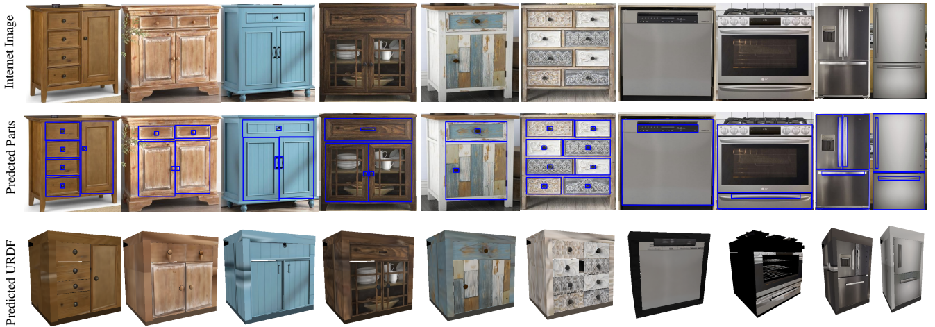
Figure 60: Reality Gym Assets: Converting real-world images into fully interactive simulation assets. Given internet images, we apply fine-tuned groundingDINO to obtain 2D part boxes. These boxes and RGB images are fed into URDFormer to generate articulated simulation assets that match the real-world structure.
