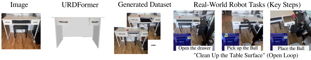
Figure 36: URDFFormer can be applied to a different robot such as a Stretch Robot to perform a multi-step task such as "clean up the table surface". We apply URDFFormer to predict the URDF of a study desk, and render a dataset to train a vision-based policy to predict an affordance map at each step.
