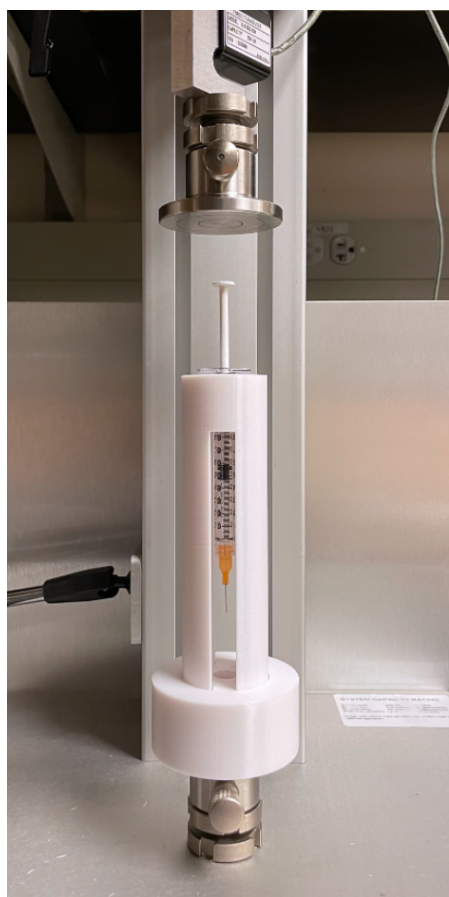
Figure C3. Custom syringe holder used for injection force measurements. It was 3D printed using fused filament fabrication, with poly(lactide) filament.
