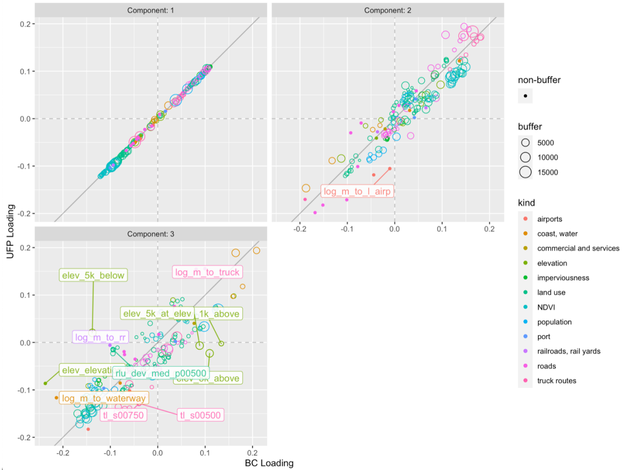
Figure 74. Comparison of UFP and BC PLS model loadings. Labeled pairs are those with the largest UFP-BC loading difference, as determined by the lowest and highest quantile from all three components ( \text{diff} < 0.1 quantile or \text{diff} > 0.99 quantile).
