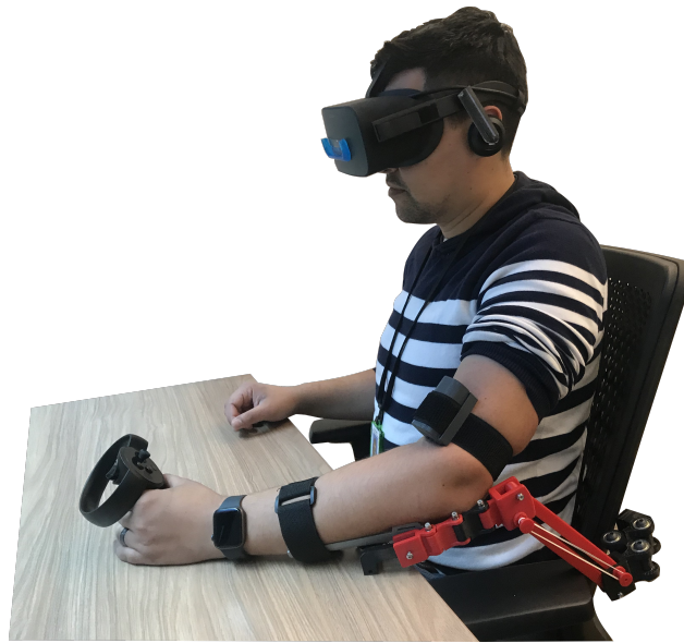
Figure 3.1: Overview of experimental setup in real life. Subject movement is tracked using a virtual reality controller and virtual targets are displayed through a headset
