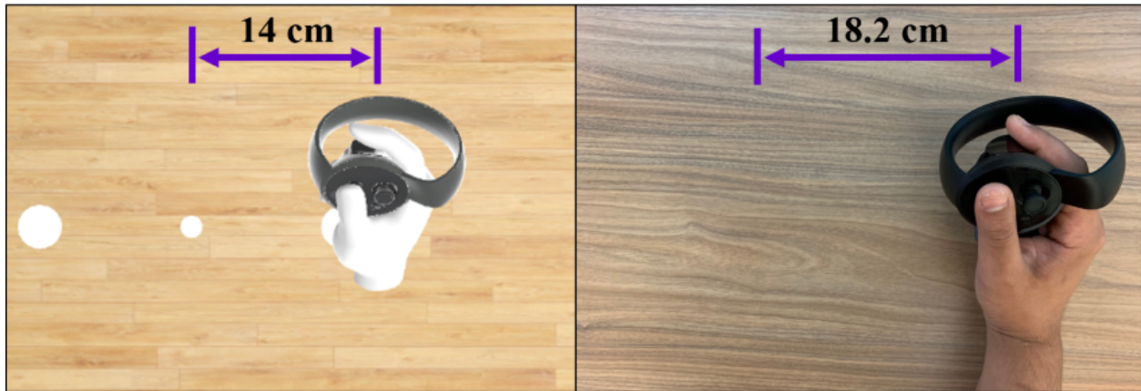
Figure 4.2: Virtual (left) and physical (right) representation of reach during induction phase under a C/D-ratio of 0.7 along the azimuth axis.
