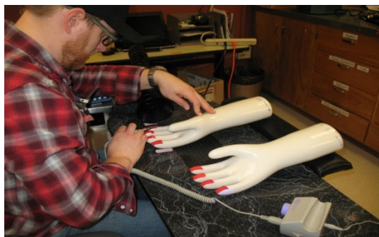
Figure 7. Nail Grinding with LEV System
