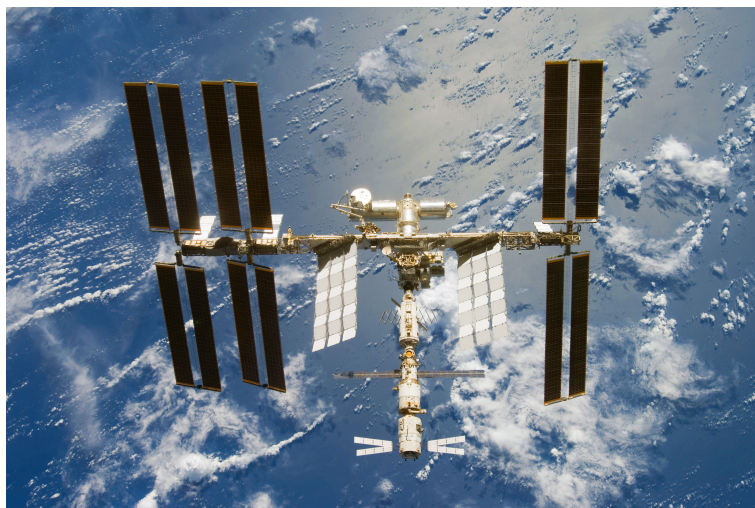
Figure 1.2: A photograph of the Automated Transfer Vehicle (bottom of image) docked with the International Space Station [9]. Other vehicles such as the Russian Progress are capable of docking at the same location.
