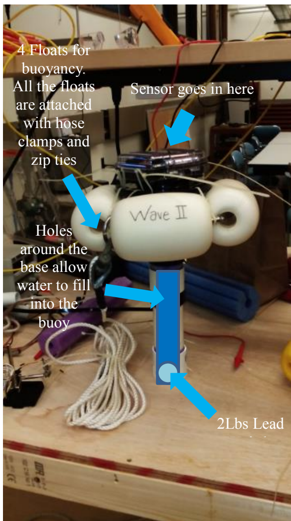
Figure 2. The final product of how everything was assembled is shown. The white rope on the left corner below the buoy will be used to attach the sensor buoy on to the large flotation buoy.
