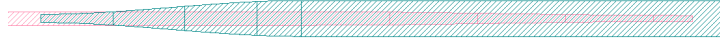
Fig. 4.11 Layout of silicon waveguide to silicon nitride waveguide coupler. Pink is silicon, and green is silicon nitride.
