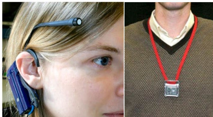
Fig. 2.13: The eye-level (left) and pendant (right) Daysimeter devices. 9
