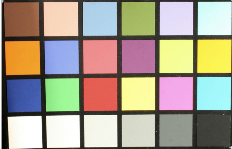
Fig. 3.10: Image of Macbeth chart under the lighting condition present at the time of image capture
