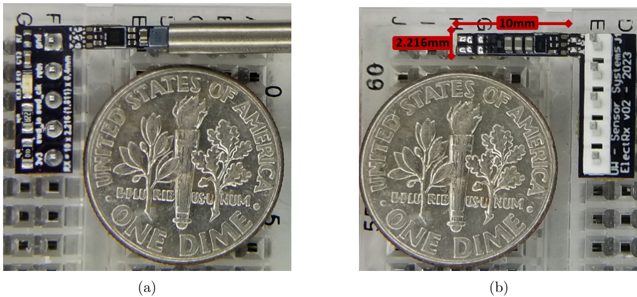
Figure 6.35: (a) ElectRX v02 Top (b) ElectRX within an 11g Needle
