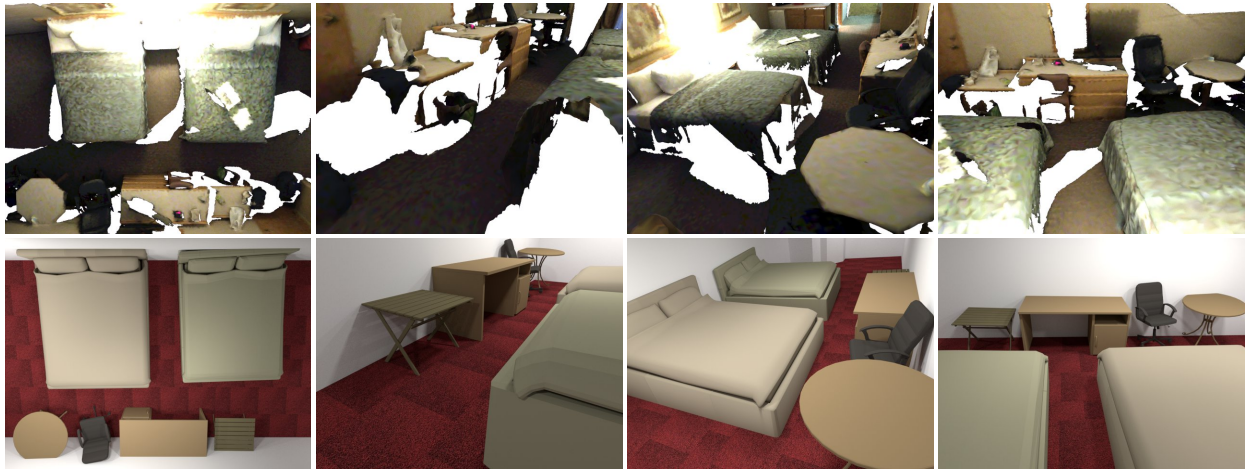
Figure 4.1: Given an RGBD sequence from a moving camera, we produce a 3D CAD recomposition of the scene. While a fused reconstruction (top) contains holes and noisy geometry, our recomposition (bottom) models the scene as a set of high quality 3D shapes from CAD databases.
