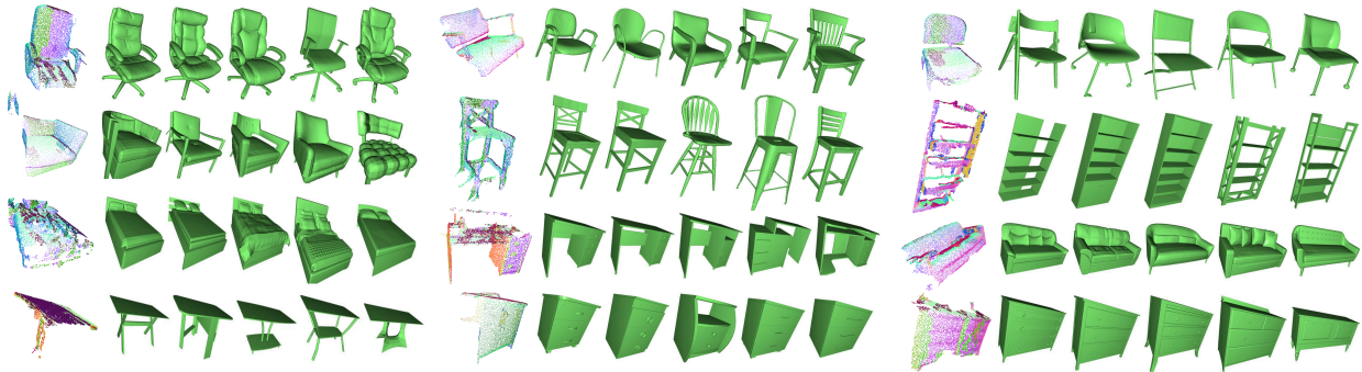
Figure 4.3: Top retrieved CAD models for each object instance segmentation as query. Point cloud query is color-coded with surface normal.
