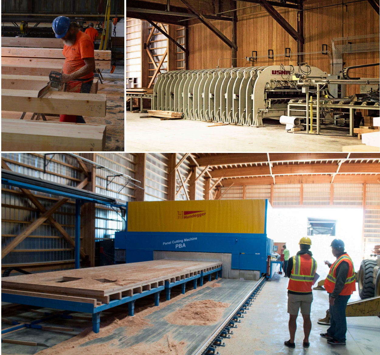
Fig 2.27: An employee adds a 'rusticated finish' to a glulam beam (left). The DR Johnson CLT press (right). DR Johnson's CNC router. (Below)
