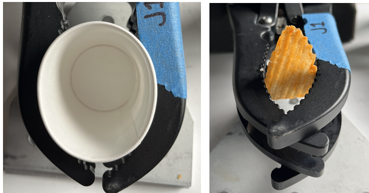
Figure 18. A paper cup (left) and potato chip (right) picture without damage after detection.
