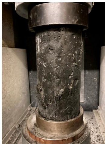
Figure 3.1: Typical compression failure
