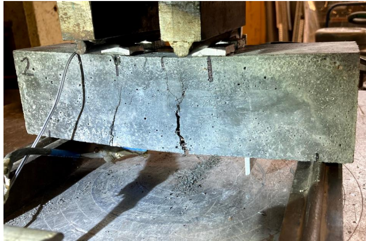
Figure A.4: Flexural beam test (a) setup, (b) typical failure
