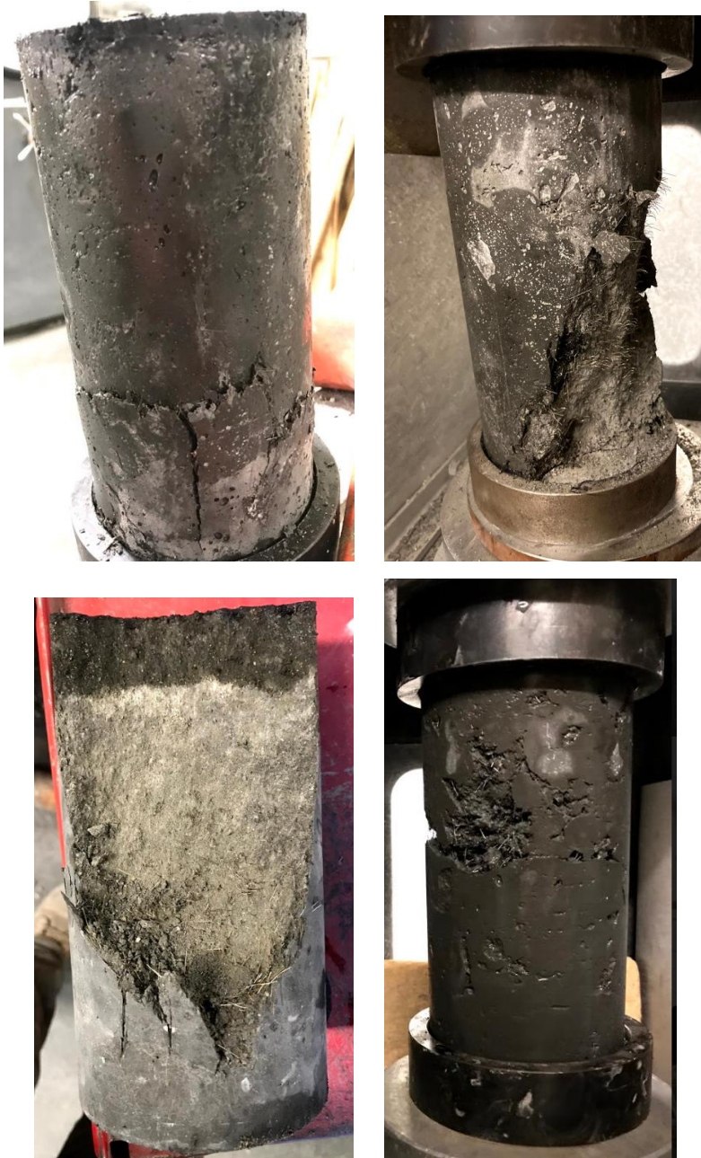
Figure A.2: Compression test (a) typical 2% failure, (b) typical 1% failure, (c) sinking fibers, (d) poor consolidation
