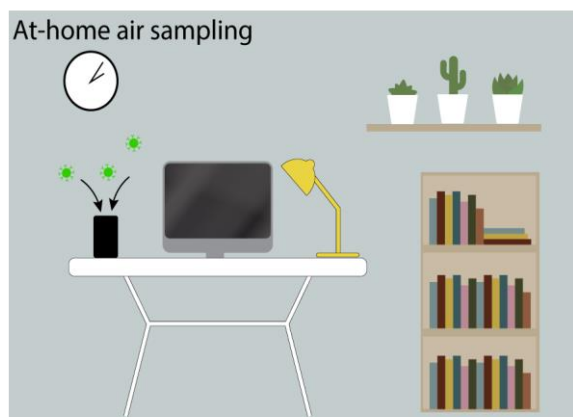
Figure 5.1. Schematic representation of our battery-powered air sampling device (small black box to the left of the computer), collecting aerosols in a home environment to provide information on the landscape of aerosols in the room. The concept is that our device can be placed in any environment (e.g., homes, schools, hospitals, playgrounds, and farms) and then sent back to a laboratory for analysis.
