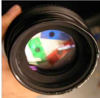
Figure 2-3 The three color-filtered pinholes on the aperture mask
