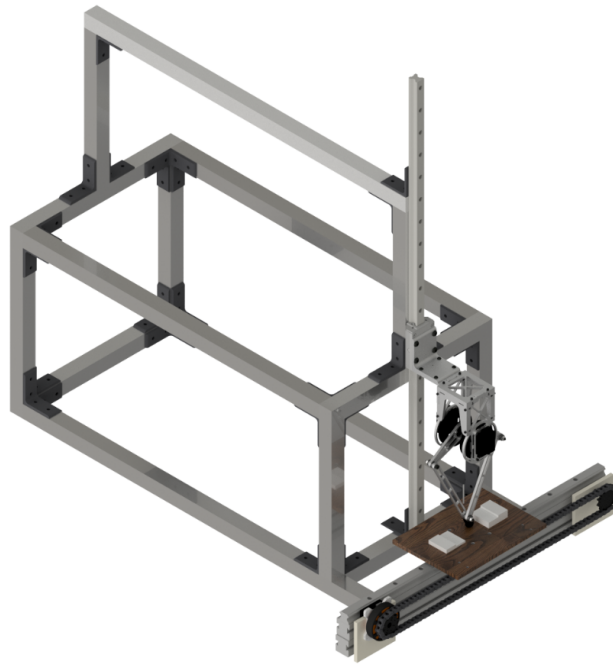
Figure 3.2: The CAD model of the test bed
